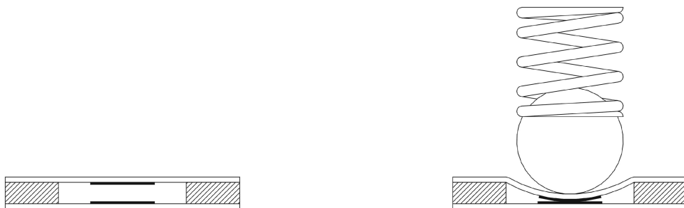
Sketch 3: Sectional view; how contact is achieved
